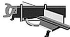
**Nail and Glue Mitres:** Trim each of the two mitring members at opposite angles. When fitted together they should form a tight right angle. For tight mitre joints, nail and glue joint. Make sure the nails are countersunk below the surface.
